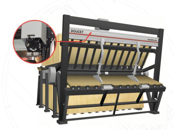
The Robotic Loosener automatically loosens the clamps holding the panels in the section above the carrier's workstation while the operator lays-up, flattens and tightens the next panels. The system also indexes the carrier forward automatically. That approach enables you to retain total control over the flattening and tightening of your panels, while reducing the time devoted to gluing panels up to 30%.
